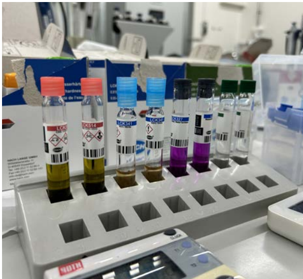
Determination of the parameters COD, nitrite, water hardness, and nitrate in raw wastewater using cuvette tests.
